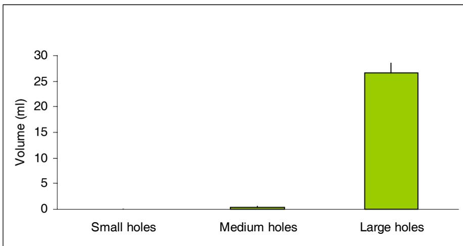
Figure 3 – Mean volume (ml) per holes of rock destroyed by the different types of macroborers on the offshore breakwater of La Spezia Gulf. Large holes are those created by bivalves. Medium by polychaetes and small by amphipods.
