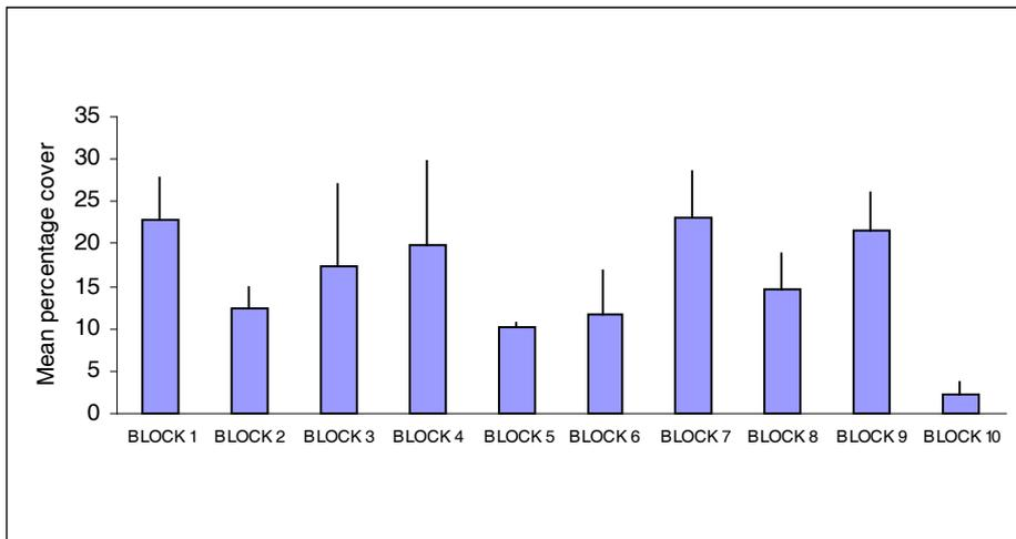
Figure 2 – Mean percentage cover of holes observed on the rock surface of each limestone blocks on the offshore breakwater of La Spezia Gulf.
