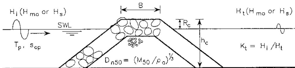
**Figure 1.** Governing parameters for wave transmission
